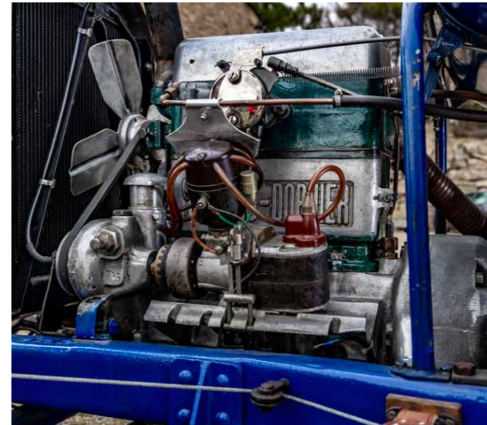
The Chapuis-Dornier CST4 1100cm2 on the admission side. Less advanced than the 12-valve model, it is also more reliable. Our example is fitted with a tailor-made exhaust pipe to gain a few more horsepower.
