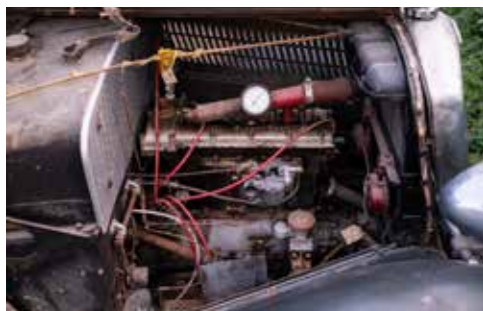
The engine installed today is an S4-DA, and has not been run since 1972.
