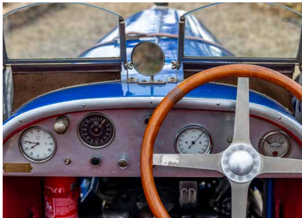
The dashboard contains the essentials: rev counter, speedometer, clock and oil pressure.
