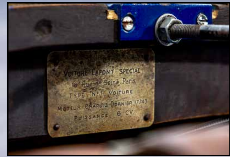
The chassis plate shows the manufacturer's address, the chassis number and a Chapuis-Dornier engine number that does not match the current one. Perhaps this is the number of the 12-valve engine originally fitted!
