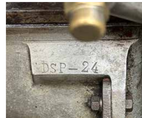
The DS Ruby engine was extensively modified by Germain Lambert. This is the «racing» version with the inscription DS «P», which Michel Piat believes could stand for «Spécial». As on the racing 16, it is probably fitted with a customized crankshaft and lighter connecting rods. Among other modifications, Germain Lambert had the crankcase castings redone so that a magneto could be fitted, a feature not possible on standard DS versions of the Ruby.
