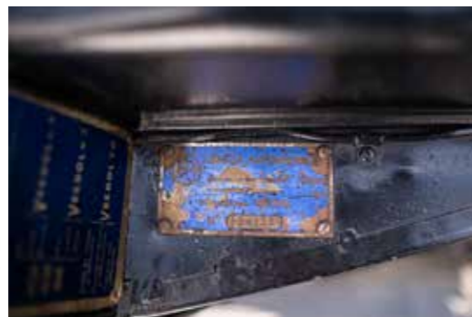
The chassis plate and the cold stamping on the self-supporting shell match.
