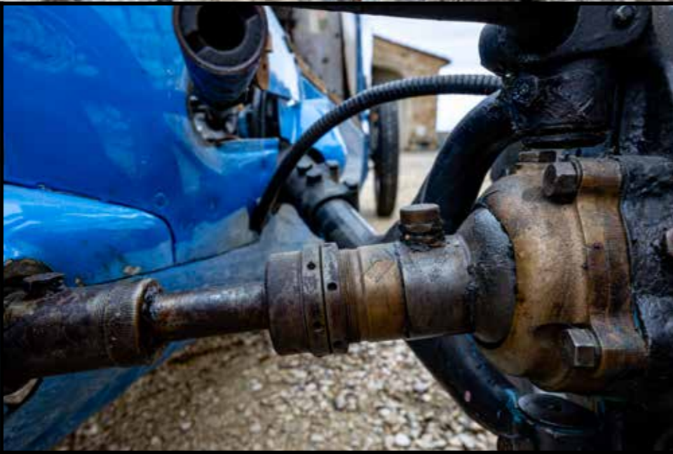
Zooming in on the traction system, the wheels are driven by half-shafts fitted with universal joints, designed by Chevallier.
