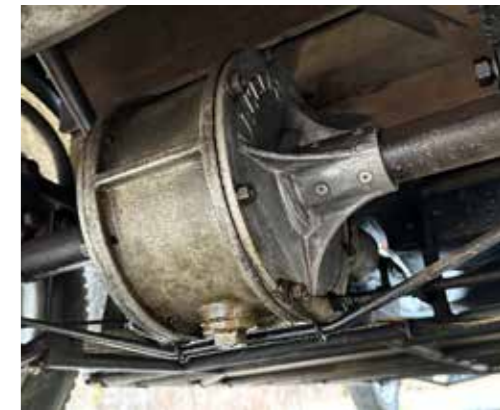
Both the bridge and the gearbox are of Lambert design, we can clearly see the inspiration of his masters Bugatti and Voisin, what is efficient is beautiful!
