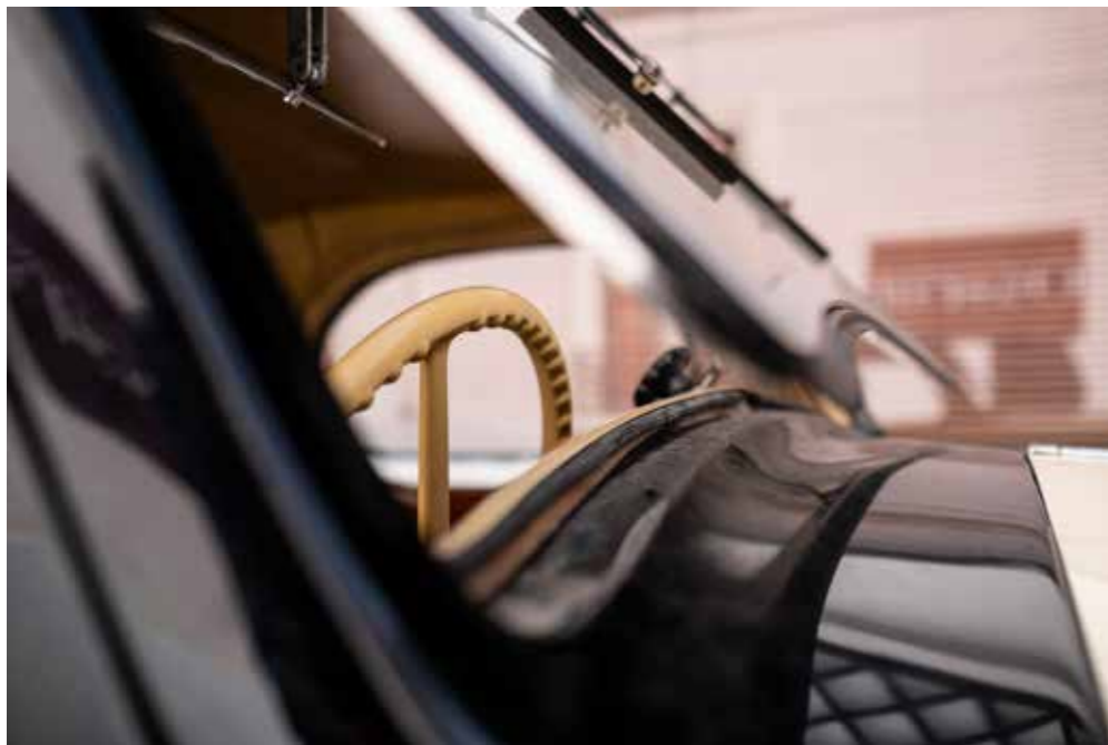
For the hot summer days in Castres, a windshield with an opening system had been installed, to ventilate the passenger compartment.
