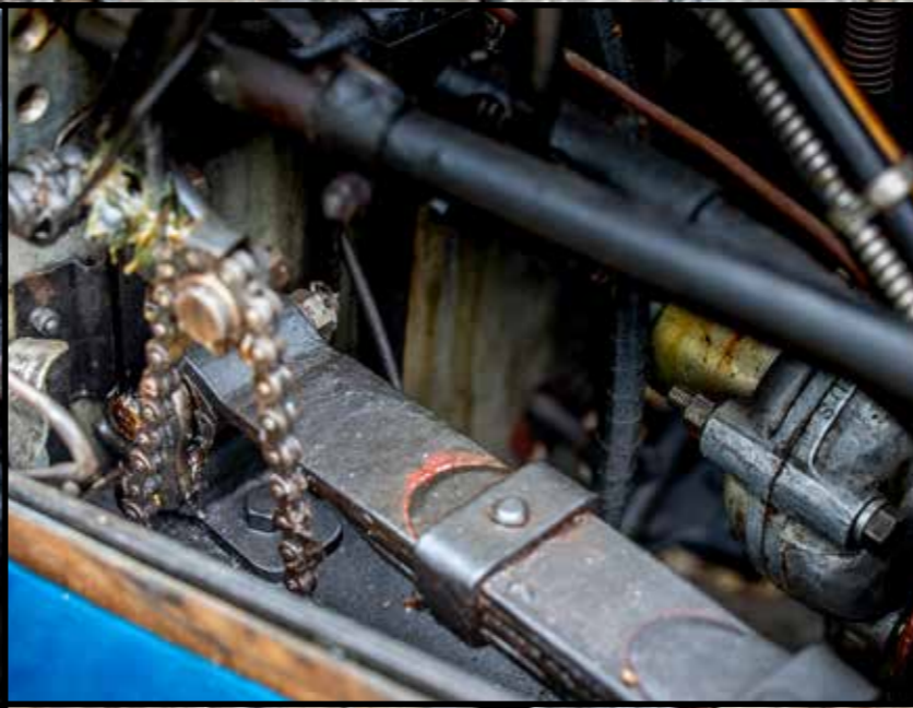
On the suspension side, each wheel is attached to a large lever arm which, on the wheel side, receives the steering pivot and universal joint by means of a fork, then articulates to the chassis by means of leaf springs. The DALILA cyclecar had already used this principle in the early 1920s, and it was later used on the 2CV.
