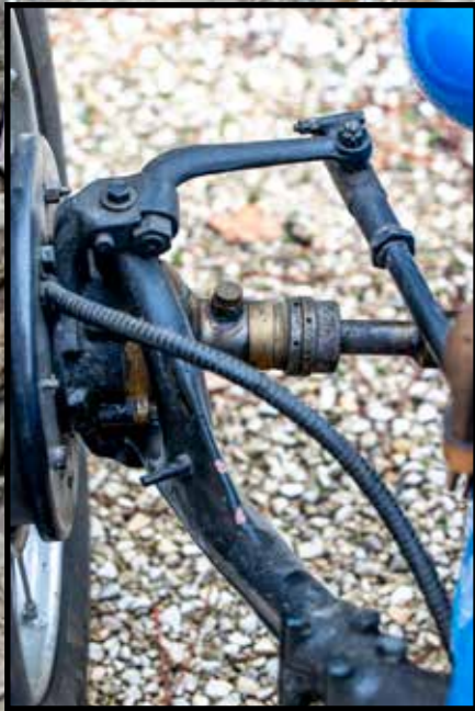
Zooming in on the traction system, the wheels are driven by half-shafts fitted with universal joints, designed by Chevallier.
