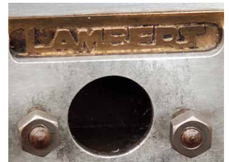
The bronze cylinder head with "Lambert" foundry.
