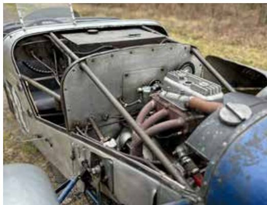
Everything for lightness. Germain Lambert understood it well, Lambert/Ruby would not be enough to win races. Tubular chassis, aluminum bodywork and hollowed-out wood and steel parts made it possible to obtain an extremely light, maneuverable and lively car despite its small engine capacity.
