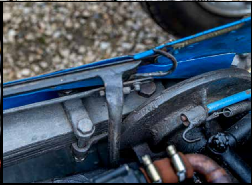
On the suspension side, each wheel is attached to a large lever arm which, on the wheel side, receives the steering pivot and universal joint by means of a fork, then articulates to the chassis by means of leaf springs. The DALILA cyclecar had already used this principle in the early 1920s, and it was later used on the 2CV.
