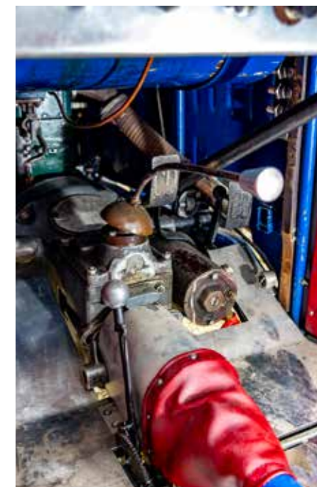
The gearbox and pedal assembly. The clutch pedal has been modified to fit a starter motor.
