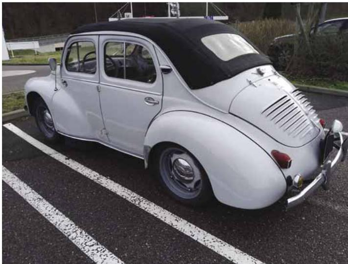
With its tumbled engine, it was a light car capable of reaching 90 km/h. Within the reach of modest pockets, the 4CV became a true symbol of freedom.
