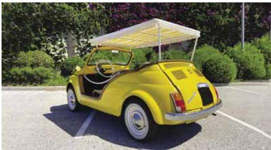
Rare model derived from the Fiat 500 made by the coachbuilder Jacques GAUCHET within the company TPLV in Paris. The particularities of this Fiat 500 are first of all the cut of the roof, the mahogany veneer all around the cockpit, and the braided rope replacing the doors. Usually a plastic cane is used for the seats, replaced here by wicker seats in the front and in the back. The car is in very good condition inside and out. Mechanically flawless, this atypical Fiat 500 will take you everywhere.
