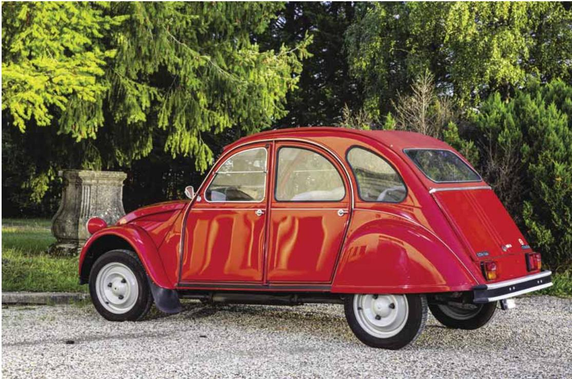
three-speed gearbox, easy to maintain, with a suspension allowing to cross a ploughed field with a basket of eggs without breaking a single one, and consuming only 3 liters per 100 kilometers! It must be easy to drive, by a beginner or a woman. And above all, no ostentatious signs. The advertising slogan "4 wheels under 1 umbrella" of the end of the 60's, summarizes rather well the general spirit of what the boss expected. The project is hidden from the Germans during the war
